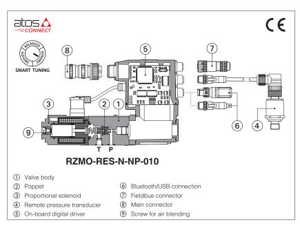
Digital proportional valves with remote pressure transducer, respectively performing: compensator, relief and reducing closed loop function.
